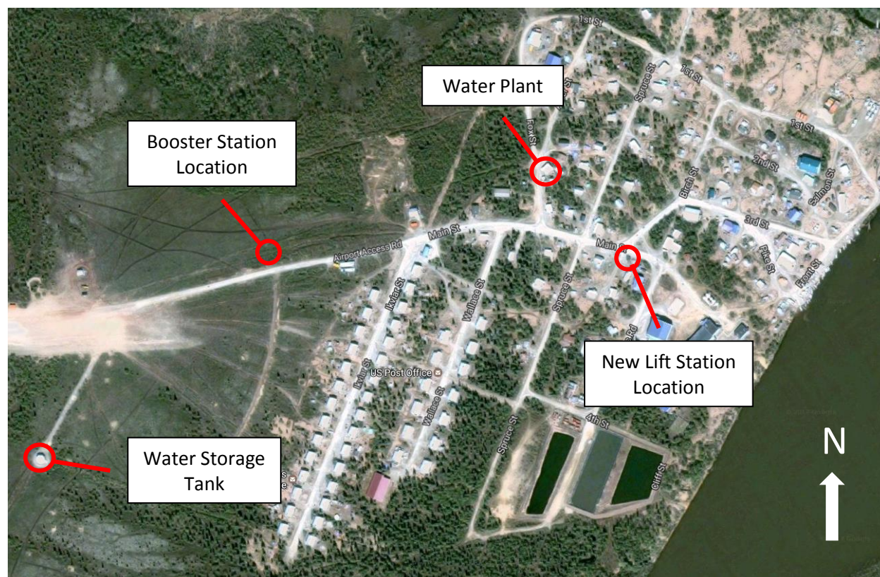
Figure 1: Aerial view of New Stuyahok, Water System Component Locations
