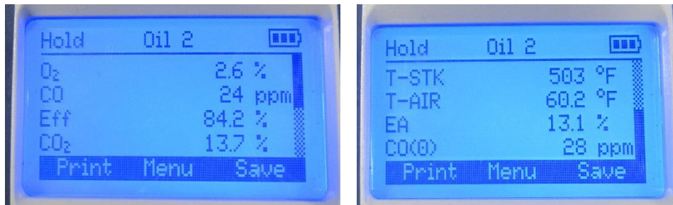
Figure 6: Boiler 2 combustion test results.
