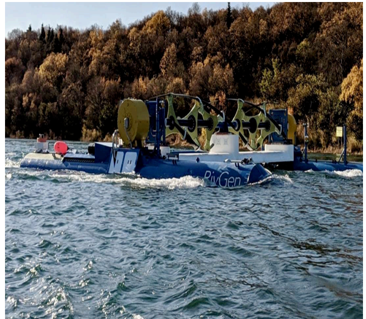
Pontoon mounted river turbine
