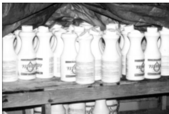
Damaged containers of chlorine (HTH) are dangerous.
