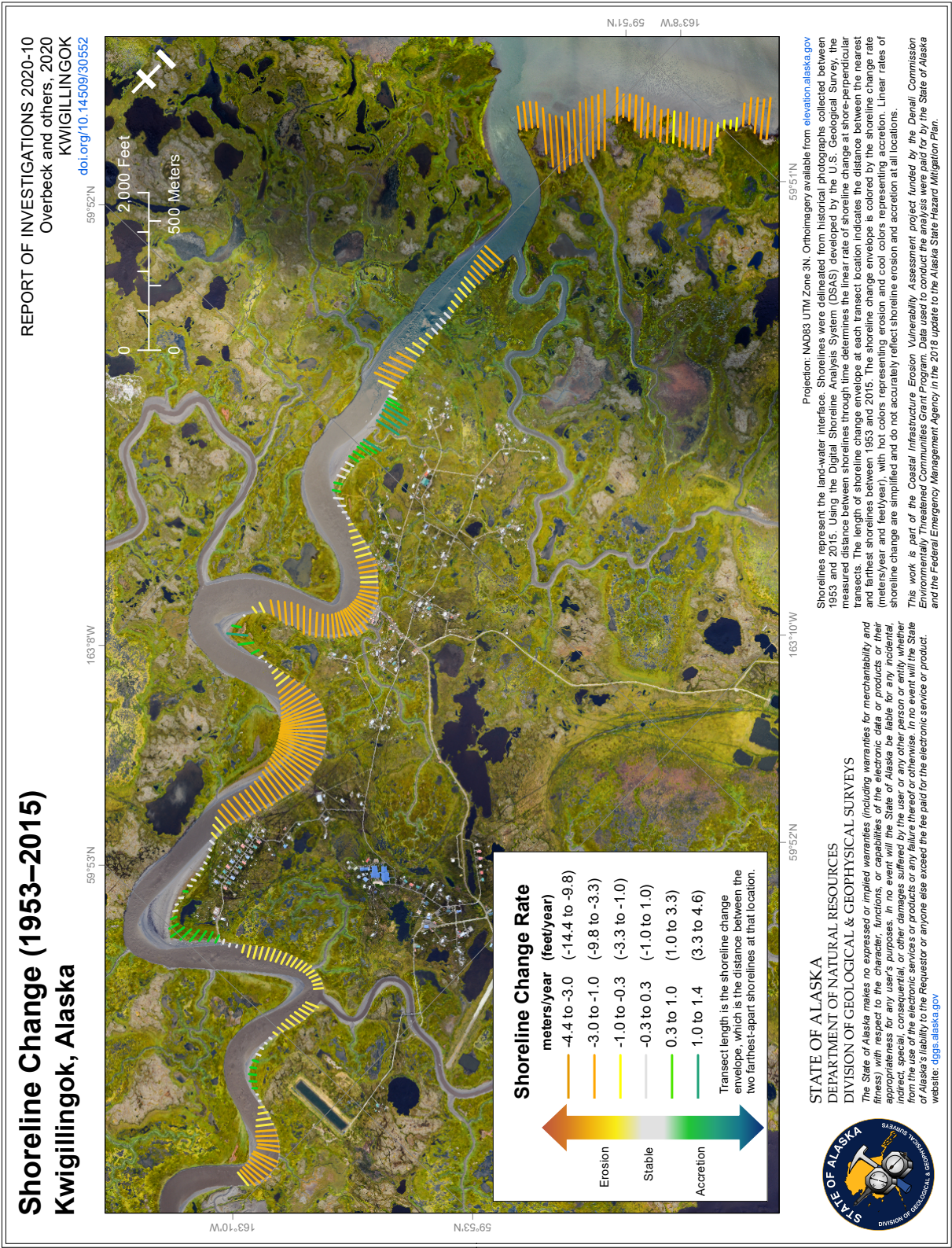
Figure 3. Example of map sheet for Kwigillingok, Alaska. Map shows the distance between the two farthest-apart shorelines at cross-shore transects (shoreline change envelope). The shoreline change envelope is colored by the rate of shoreline change, with hot colors indicating erosion and cool colors indicating accretion. Both erosion and accretion along the Kwigillingok River and erosion of coastline along Kuskokwim Bay (right side of map) have occurred (or were measured) in Kwigillingok
